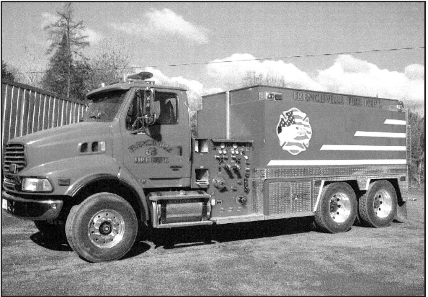
Frenchville, Maine: 2007 Sterling — Allison 4000 EVS - 3050 Gallon Water Tank — Class 1 Gauges —Akron Brass Control Handles — Gold Leaf Lettering with Black Outline — LED Lighting.
